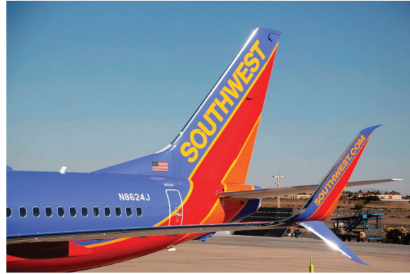
New Split Scimitar Winglets (first installations began in 2014); fuel savings of about 5.0 to 5.5 percent per aircraft.
