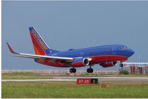
Blended Winglets (first installations began in 2007); fuel savings of about 3.5 percent per aircraft.
